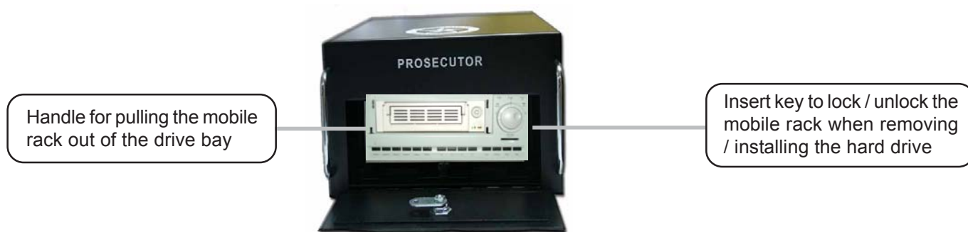
Figure 1: Removing Hard Disk
